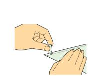
**3** Peel the cutoff section of the backing from the laminate
