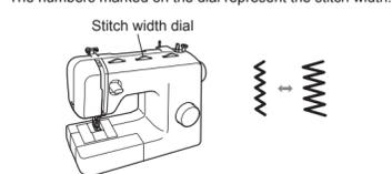
When the Straight or Triple Stretch Stitch is selected, the needle position can be changed from left to right by adjusting the stitch width dial.
