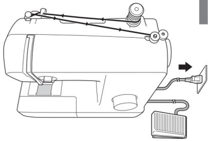
1 Pull up the spool pin completely.
