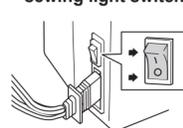
Press the power switch toward the "I" mark to turn the main power and sewing light on. Press toward the "O" mark to turn off.
