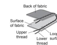
**Solution:** Reduce the tension by turning the upper tension control dial to a lower number.
