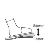
Press the foot controller down to start sewing. Take your foot off the foot controller to stop sewing.
