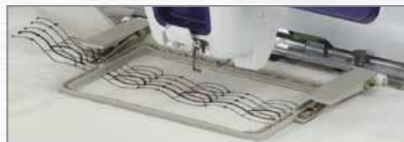
The VR offers a 180 mm × 100 mm sewing range
