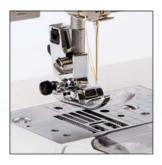
Automatic electronic needle threading
